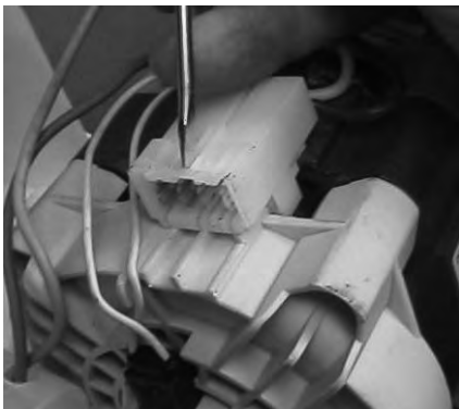
LOCK FOR DISCONNECT – FIGURE 50
