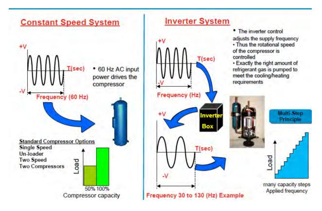
The constant speed compressor that we are used to working with is either on at full power or off. The inverter compressor will slow down as it gets closer to the set point. This gives it a longer run time at much lower power consumption. The longer run time also gives better temperature control and humidity control.
