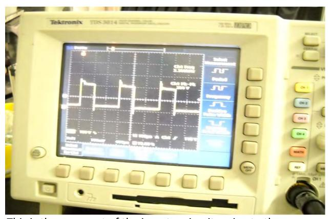
This is the wave out of the inverter circuit, going to the compressor. Notice it is a square wave. As it is a wave, it will have a frequency that can be controlled by the inverter. The following is the compressor wave form with the signal to the electronic expansion valve added. As was stated earlier the two signals have to be perfectly synchronized. The only difference you can see is a voltage difference.
