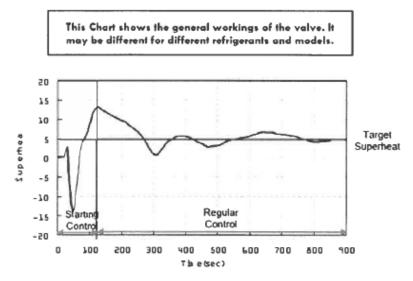
When the unit first starts, the board is receiving information from the thermistors. There is a short time that the expansion valve will appear to hunt. As the system settles the valve will become more stable. Then depending on model, it will only reposition every four or six minutes.
