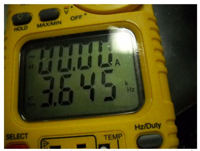
Frequency can be read on a standard meter by going on any of the three compressor leads and reading to ground. Most of our meters have a frequency scale, we have not had the reason to use it previously.
