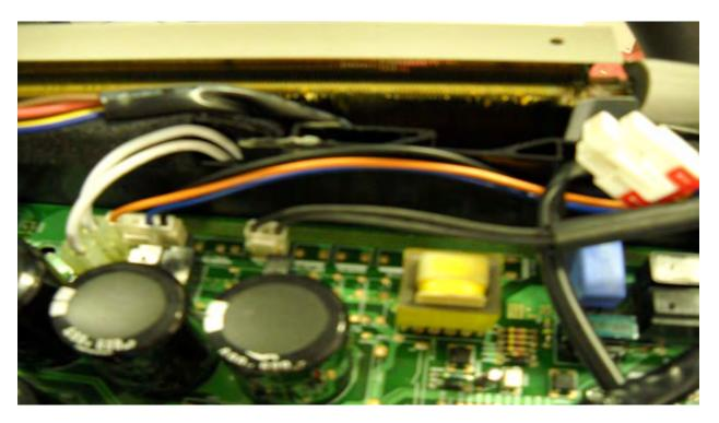
Each component that plugs into the board will either have a unique size of plug or a different color. It is difficult to miss wire these boards.
