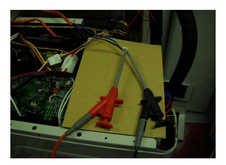
These thin spring wire leads will fit into the plug opening and also make contact with the metal on the side of the plug. Being able to clamp them on, it leaves both hands free to adjust the meter.
