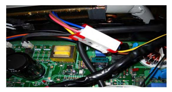
The outdoor fan motor uses a 6pin connector. If we open this connector, on the board side we can check for power. If we disconnect power we can check between the yellow and brown wire and read our capacitor. The windings of the motor can be checked on the receptacle side of the connector.
