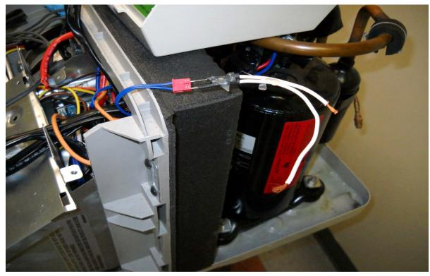
Thermistors can be checked by reading ohms or DC volts. The most common method used to check ohms. Once you have obtained the ohm reading, you can go to the thermistor chart and determine the temperature at the sensor of the thermistor.
