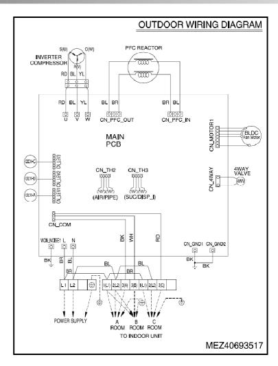
Many of our wiring diagrams simply show where to plug each component into the main control board. Most of our troubleshooting will be at the control board. It will consist of removing a plug from the board and checking the component, and on the other side checking the output of the board. If the component does not plug directly into the board, we may go to the plug for that component and do our check there.
