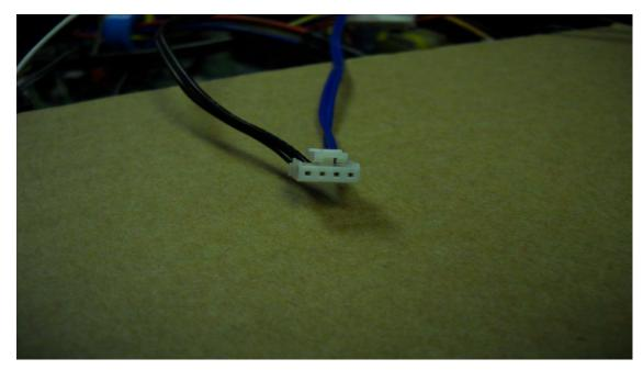
The thermister plugs have very small openings making it very difficult to take readings with normal meter leads.
