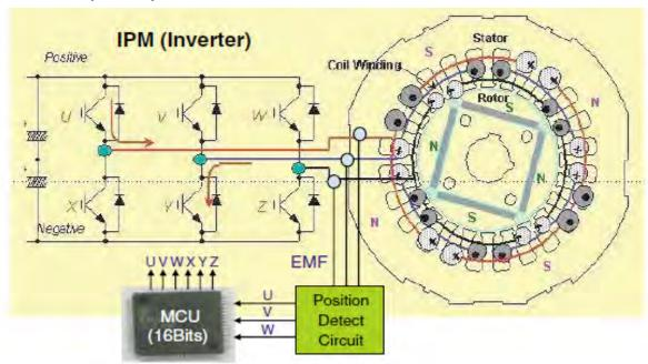
This picture shows just the bank of transistors feeding the windings of the motor.
