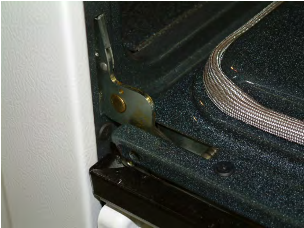
New oven door hinge and door removal
