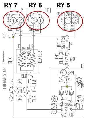
**Testing Main PCB power** output to Heating & Motor circuit.
