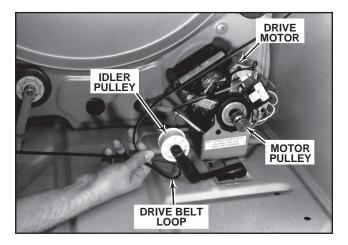
When assembling the belt on the motor pulley, first form a small loop, then slide the drive belt under the idler pulley. Push the idler assembly to the right, and at the same time place the loop of the belt over the end of the motor pulley.
