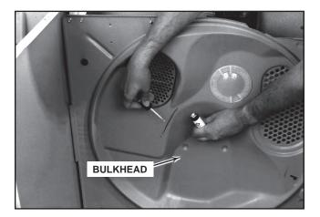
This bulkhead also supports parts of the heat and air systems.
