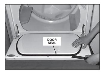
When replacing this seal place a bead of silicone rubber adhesive/sealant around the groove in the rear door panel. Place the door seal with the round side in the groove in the rear door panel.
