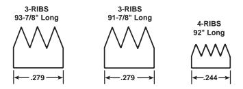
Belt "Vees" must fit evenly into the grooves on the motor pulley. If the "Vees" are out of the grooves, higher-than-normal drum speeds will be attaind, causing the clothes to cling to the drum sides, resulting in prolonged drying time or excessive wrinking of clothing.
