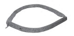
When replacing this seal, make sure the folded edge of the seal is facing away from the front cabinet panel and the two holes in the bearing fit over the two rubber plastic clips. Reduced air pressure in the drum during operation draws the seals in and effectively seals the drum ends.
