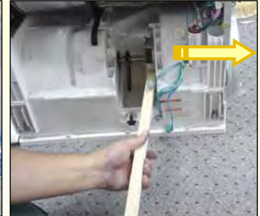
Remove drum motor
