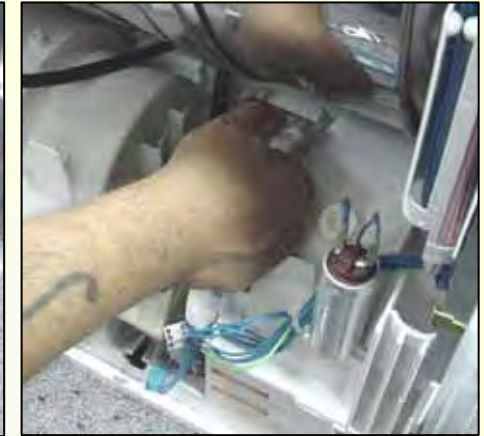
Pull out motor clamp
