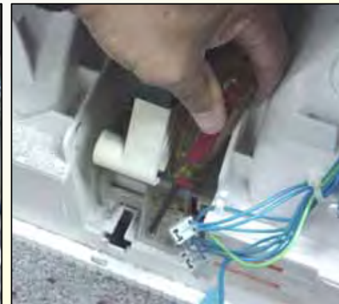
Unscrew pump cover screw
