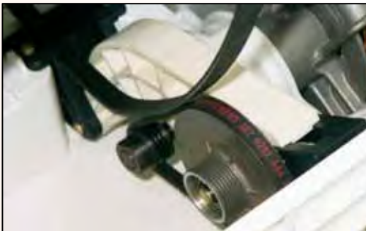
Replacing drive belt
