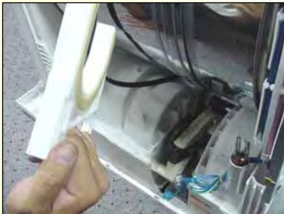
Drum motor clamp removed
