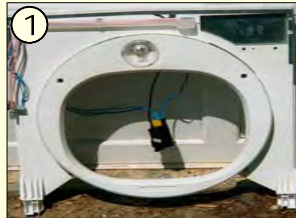
Frame with fascia, front & side panels removed.
