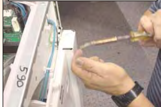
Removing front panel screws
