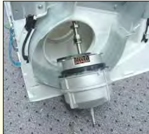
Disassembled drum drive motor
