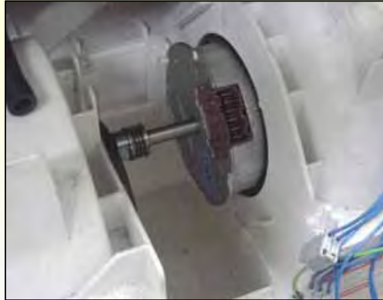
Exposed drum drive motor
