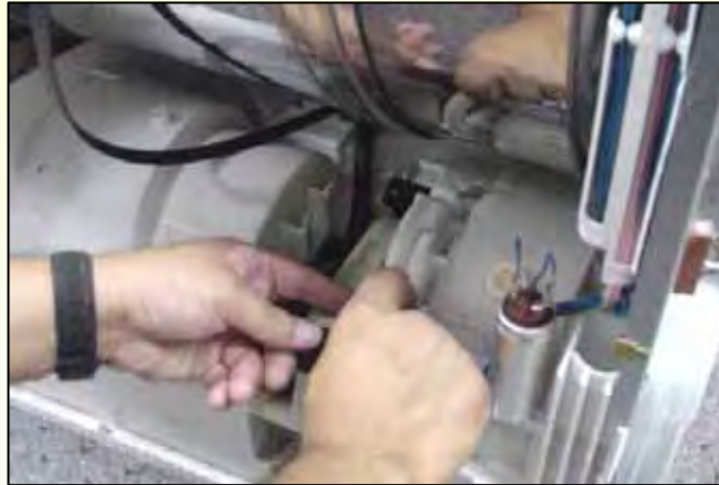
Slide drive belt off pulley
