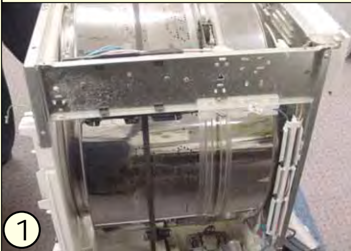
Frame with fascia, front & side panels removed.
