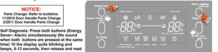
Forced Mode: Press both buttons (Energy Saver- Fridge) simultaneously (No sound when both buttons are pressed at the same time) 'til it beeps and goes blank, 8-12 seconds.
