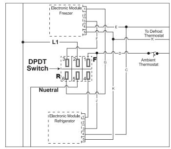
Figure 3-3. DPDT Switch Arrangement
