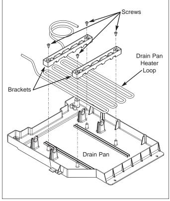
Figure 5-27. Drain Pan Heater Loop Removal
