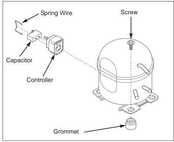
Figure 5-26. Compressor Components
