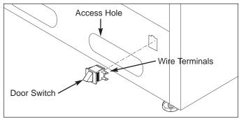
Figure 5-10. Door Switch Removal
