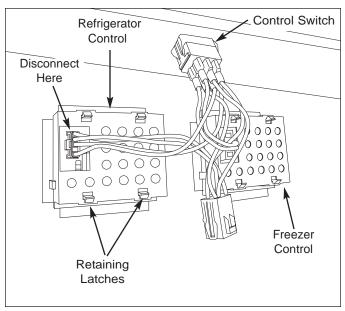
Figure 5-18. Removing Electronic Control Components Viewed From the Inside of the Evaporator Panel
