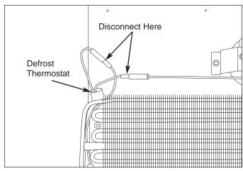
Figure 5-20. Defrost Thermostat Removal
