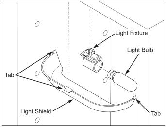
Figure 5-14. Light Shield and Fixture Removal
