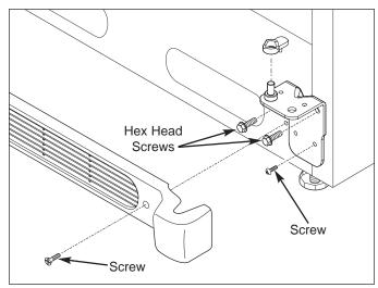
Figure 7-5. Bottom Hinge Removal
