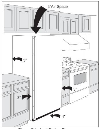
Figure 7-1. Installation Clearances
