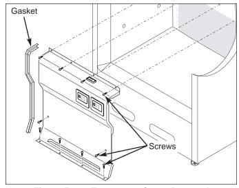
Figure 5-16. Evaporator Cover Removal
