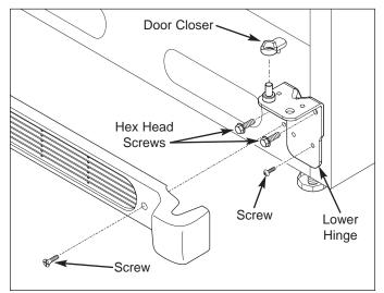
Figure 5-4. Lower Hinge Removal
