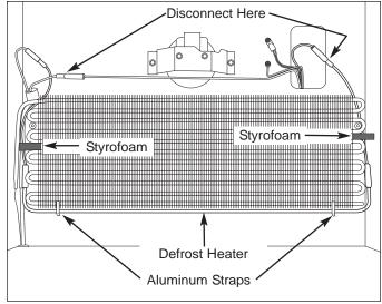
Figure 5-21. Defrost Heater Removal
