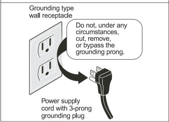
Figure 7-3. Electrical Receptacle
