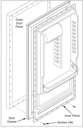
Figure 5-6. Inner Panel and Door Gasket Removal
