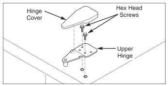
Figure 5-3. Upper Hinge Removal
