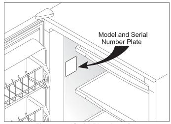
Figure 1-6. Serial Plate Location
