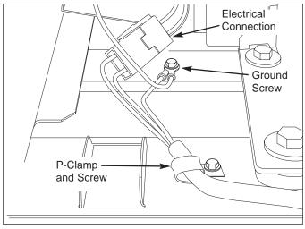
Figure 5-23. Power Cord Removal
