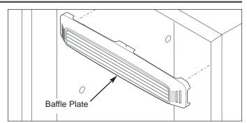
Figure 5-15. Baffle Plate Removal
