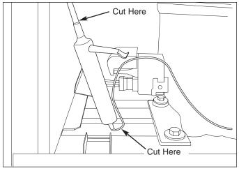
Figure 5-24. Filter-Drier Removal
