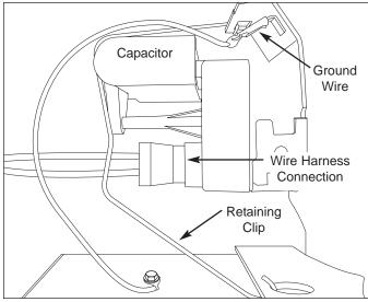
Figure 5-25. Compressor Electrical Component Removal
