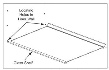
Figure 5-11. Glass Shelf Assembly Removal
