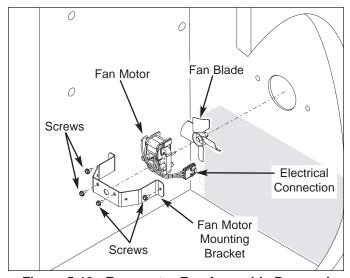
Figure 5-19. Evaporator Fan Assembly Removal
