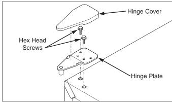
Figure 7-4. Top Hinge Removal
