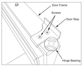
Figure 5-5. Door Stop Removal
