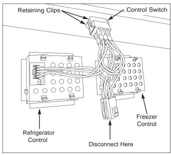
Figure 5-17. Electronic Control Components Viewed From the Inside of the Evaporator Panel
