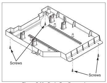
Figure 5-28. Drain Pan Removal
