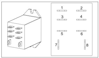
Figure 3-4. Fan Relay Terminal Arrangement
