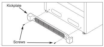
Figure 5-2. Kickplate Removal
