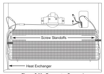
Figure 5-22. Evaporator Removal
