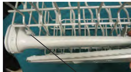
Retainer on rear of center arm delivery tube
