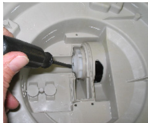
Forcing motor from sump
