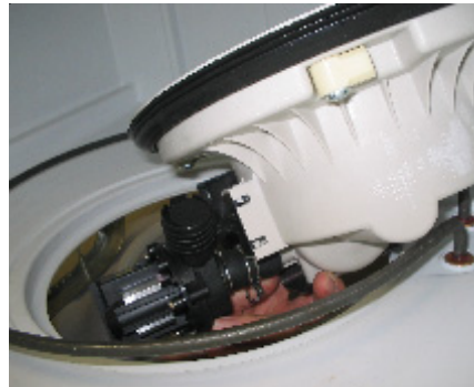
Lift sump to the 2:00 position to remove
