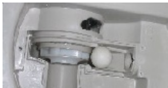
Check ball moved up ramp.
