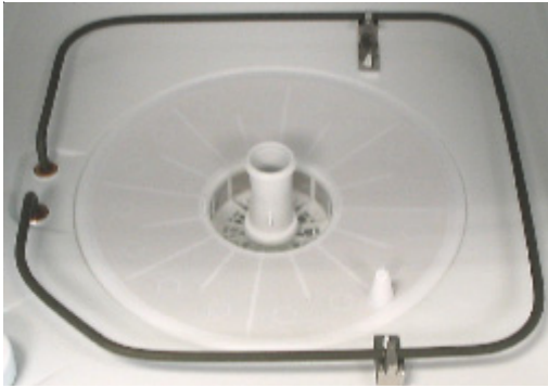
Heater for the Precision wash system
