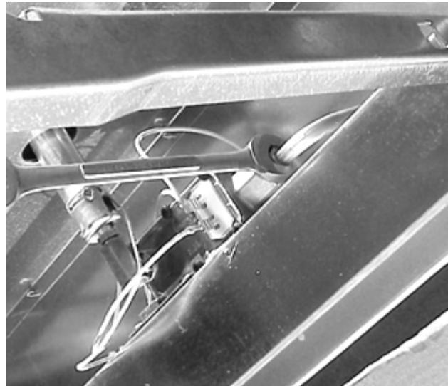
Disconnect tubing from front
