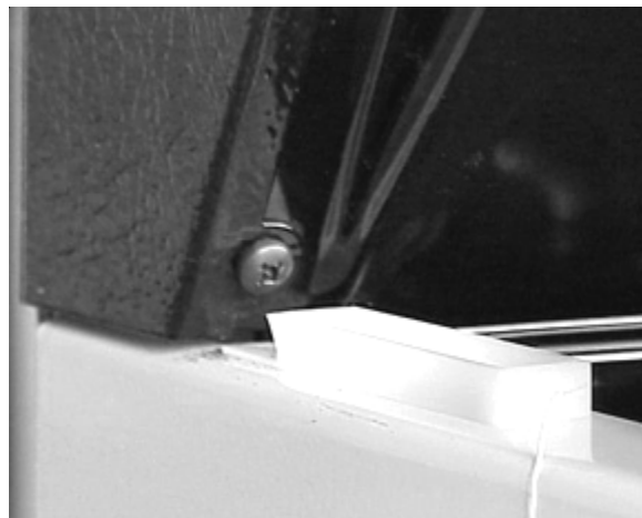
Backguard screw in each corner
