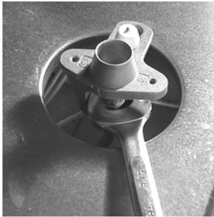
Removing burner base
