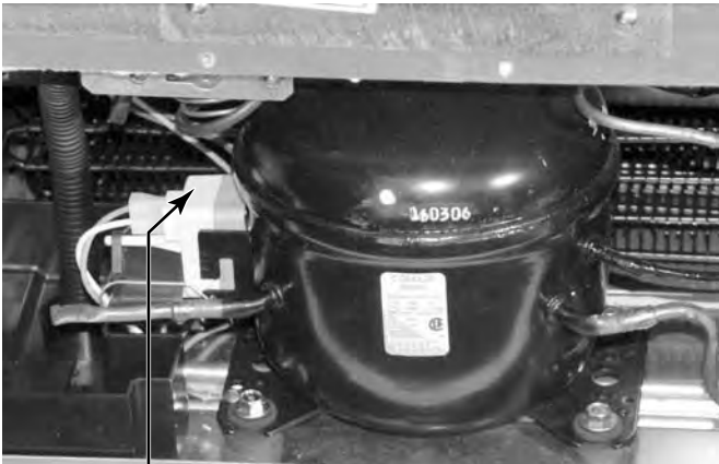
Remove the Run Capacitor and Relay / Overload
