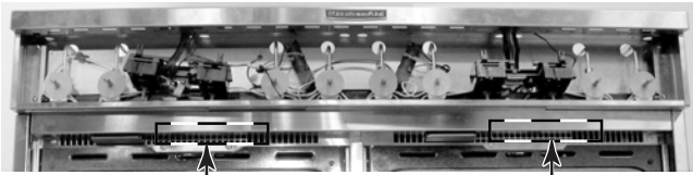
Control Panel Thermal Fuses (Behind Vent Grille)
