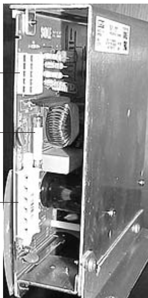
10 PIN PLUG (C 10) SPEED CONTROL BOARD FUSE (See NOTE Page 52) 6 PIN PLUG (C 6) SPEED CONTROL BOARD
