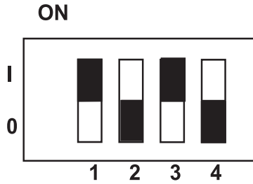
CORRECT SWITCH SETTINGS FROM FACTORY
