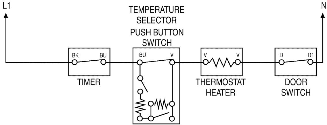
4. **Electric Heater Element Circuit - Heater element ENERGIZED.**
