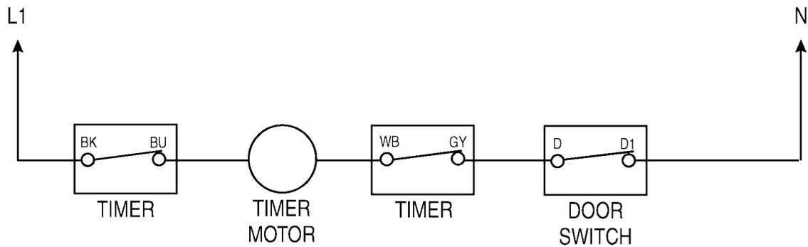
10. **Timer Motor Circuit - Automatic dry cycle.**
