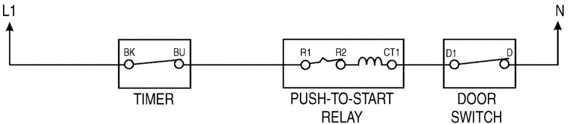
7. **Buzzer Circuit - Timer contacts OPEN**
