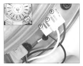
Normal resistance is approximately 11.6.0  $\Omega$  between any 2 pins (1,2 or 3) on motor
