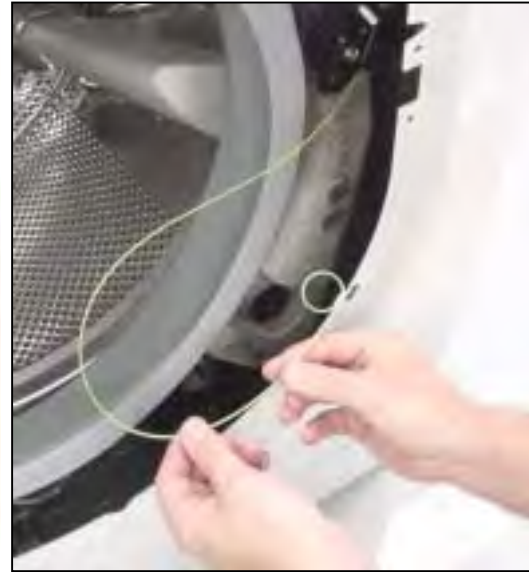
Note door latch manual release
