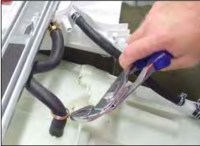
Disconnect dispenser hoses
