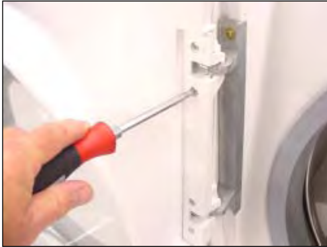
Remove hinge cover screws
