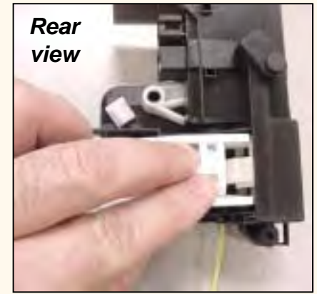
Push onto back of door lock until it clicks open
