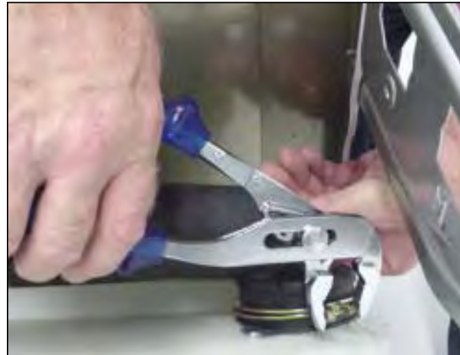
Disconnect main water inlet hose
