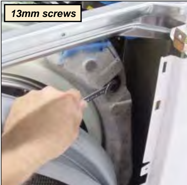
Remove right and left front counterweight screws
