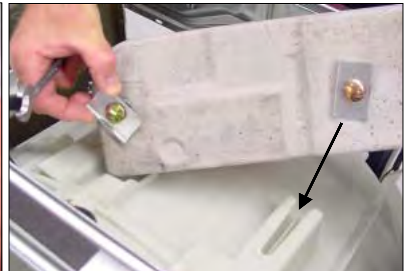
Note top counterweight bushing slots in tub
