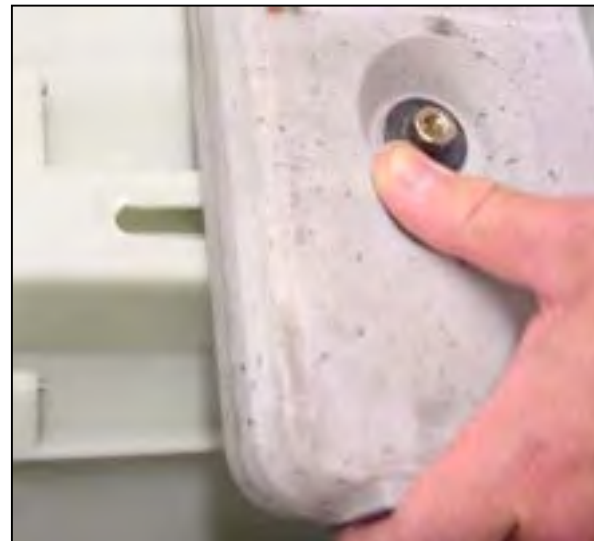
Slide out top counterweight
