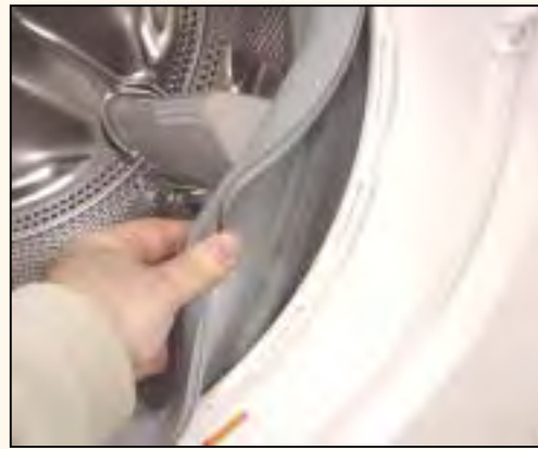
Move door seal for access
