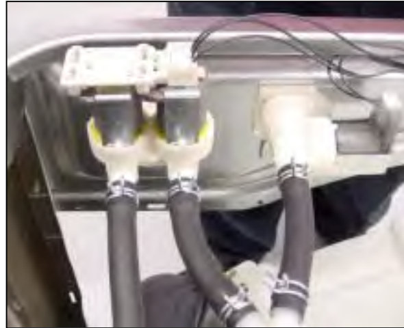
Disconnect water inlet valve hoses
