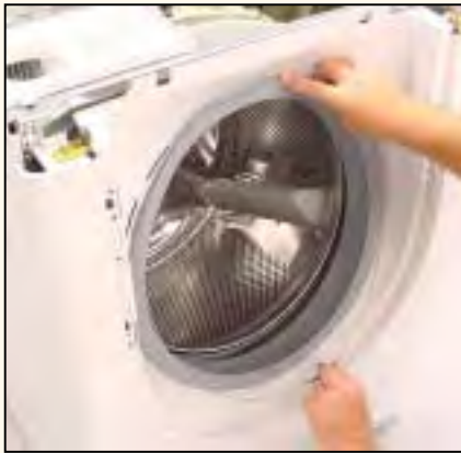
Remove front seal spring
