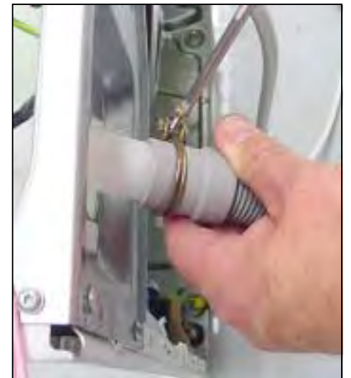
Disconnect drain hose
