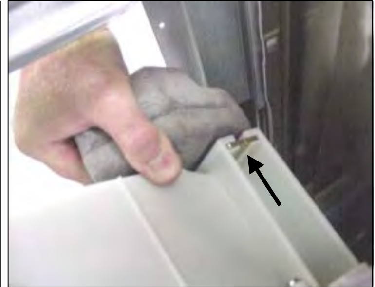
Note counterweight screw bushings in tub
