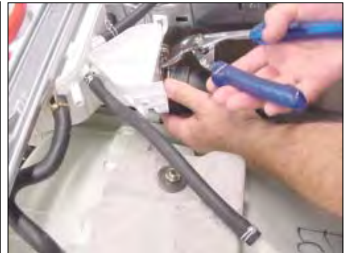
Disconnecting main water inlet hose
