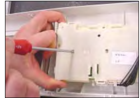
Pry out (3) inner tabs + all outer tabs
