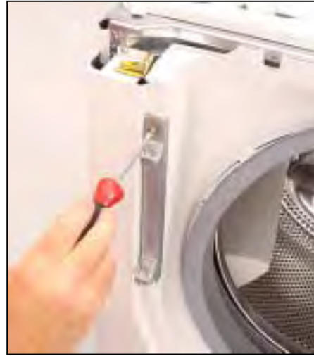
Remove hinge screws
