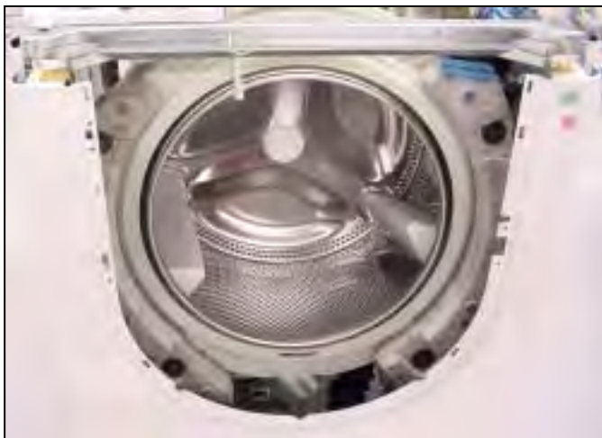
Remove front panel
