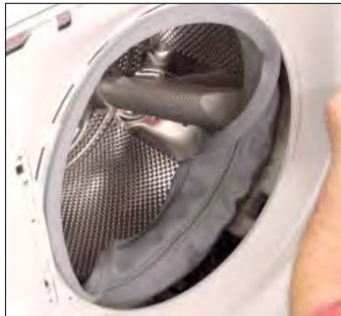
Carefully remove front shield
