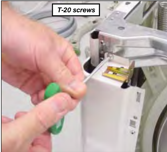
Remove top front panel screws
