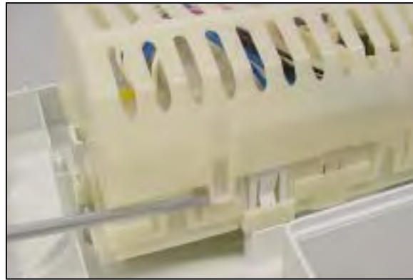
Pry outer & inner tabs together L – R
