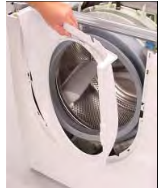
Removing front shield
