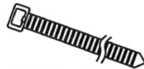
Tie strap (Option) to secure drain hose to standpipe, inlet hose, or laundry tub
