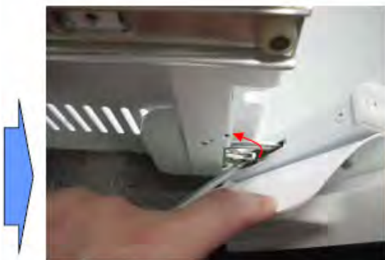
With a small screwdriver, lift lever ② from lever ③ to engage lever ①.
