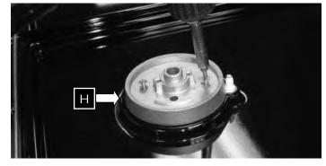
Remove each of the stack burner heads.
