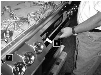
Remove all of the screws that hold the channel support G to the cooktop chassis. Lift the channel support out of the chassis.
