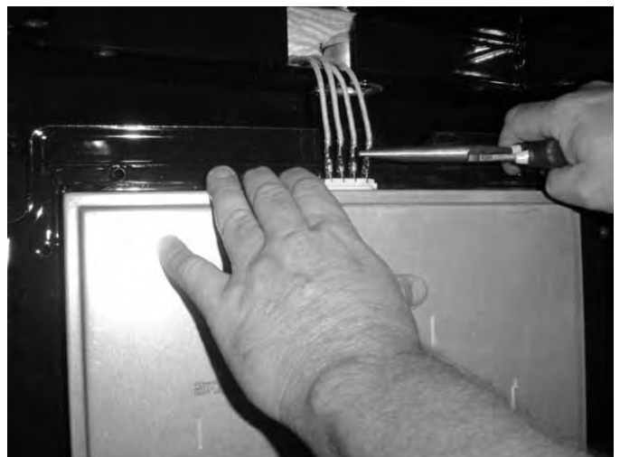
Connecting the Broil Element Wires
