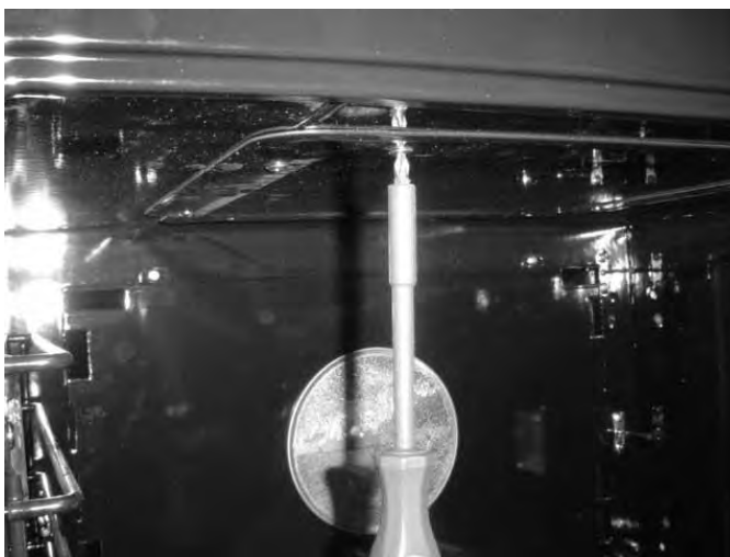
Broil Element Removal
