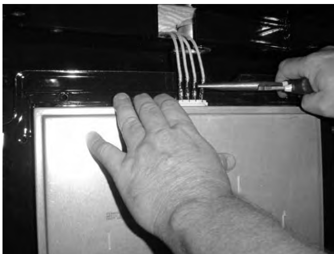
Broil Element Terminal Block
