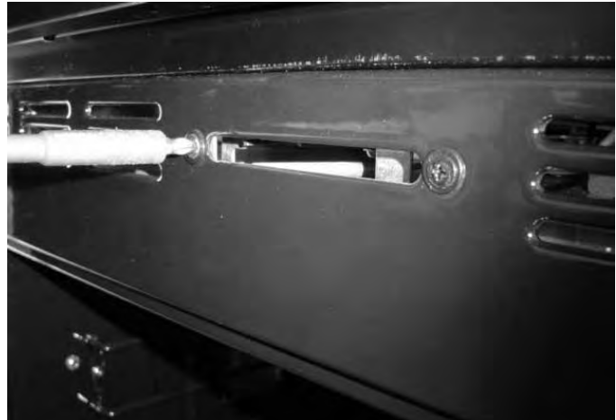
Lower Door Latch Screw Locations
