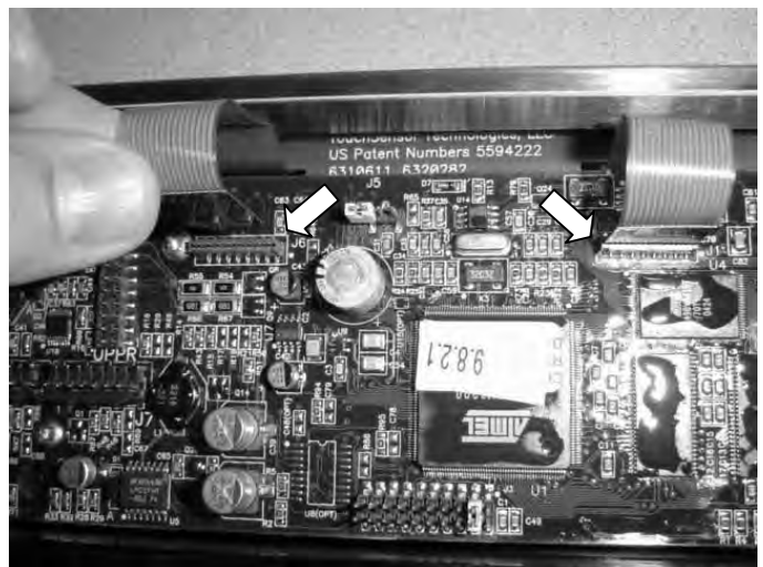
Display Flex Connections
