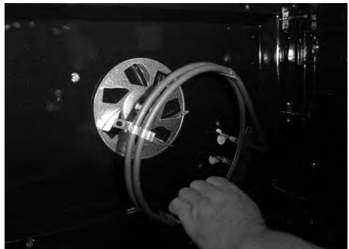
Convection Element Removal
