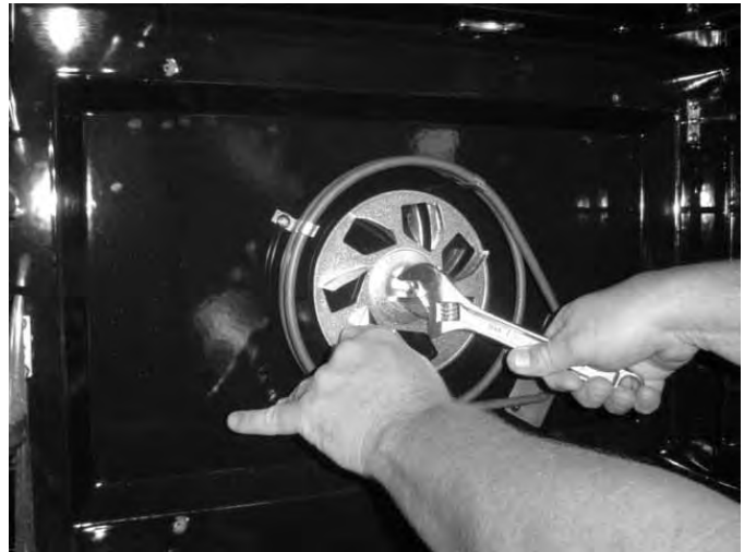
Convection Fan Nut Removal
