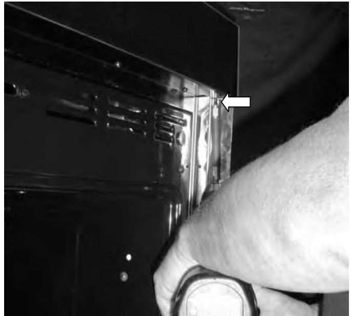
Control Panel Trim Post Screw Location
