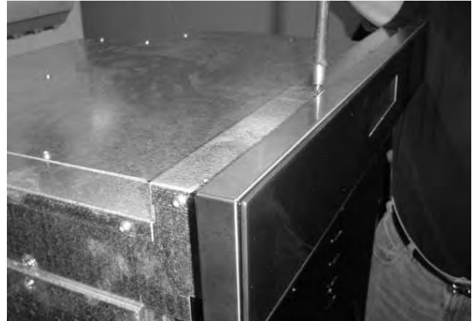
Screws on Top of Control Panel
