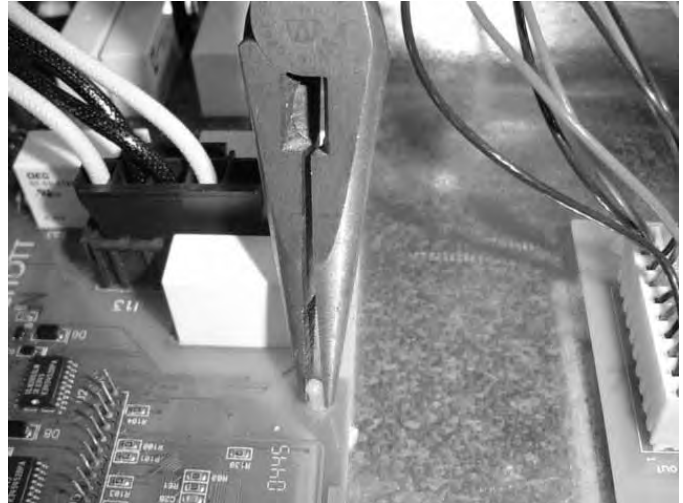
Circuit Board Removal
