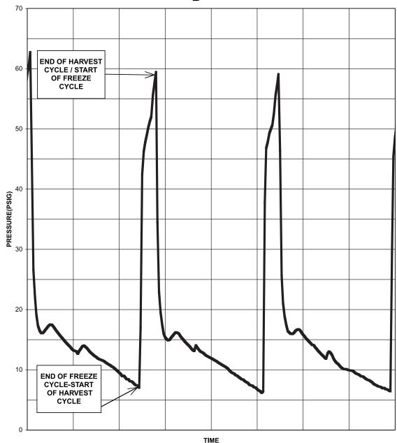
The chart above shows the low side pressure changes through the cycles of a CLR6O unit. It shows that during a harvest cycle, the low side pressures climb to nearly 6O psig. When the freeze cycle starts, the pressure quickly drops to approx. 17 psig and throughout the freeze cycle it continues to slowly drop to approx. 7 psig just before the harvest cycle.
