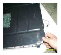
3. Dissemble the lampshade from the low lid, and loosen the screws fixed the LED light.
