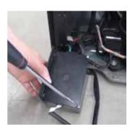
3. The main control panel is fixed in the panel box by a screw, dismantle it ,the control panel will be removed
