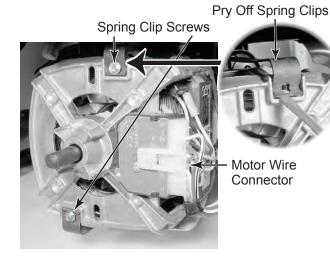
f) Pull the motor away from the washer until the motor coupler pins disengage from the motor coupler isolator, and remove the motor.
