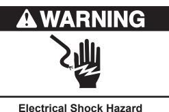
Disconnect power before servicing. Replace all parts and panels before operating.
