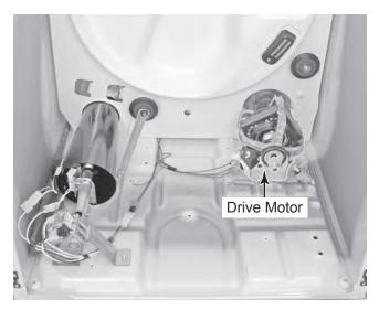
5. Lift the top tab, and disconnect the wire harness connector from the drive motor.
