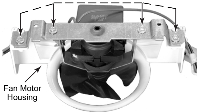
4 Evap Fan Motor Rear Bracket Screws
