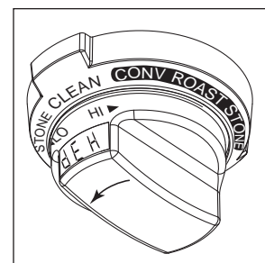
Figure 3-40. Turn and Hold Knob to Left Until “deH” Appears In Knob Display and Release Knob
