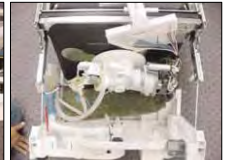
Pulling base carefully from tank & sump
