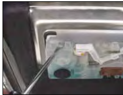
Bending retainer tabs
