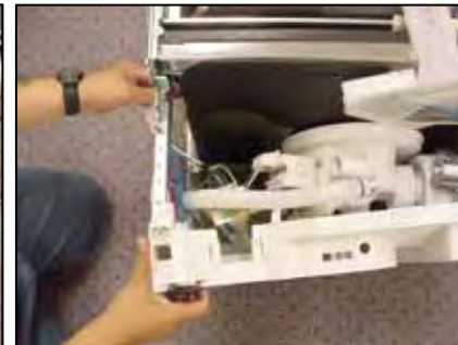
Pulling base carefully from tank & sump
