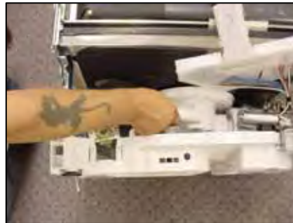
Pulling out sump hose
