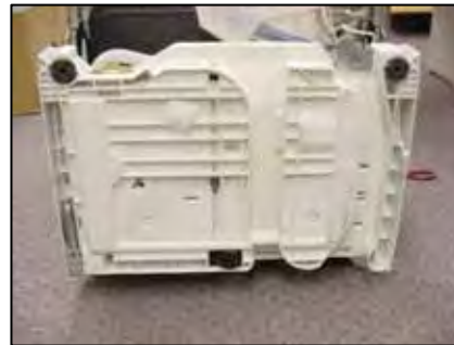
Pulling out door springs from base & disconnecting cords
