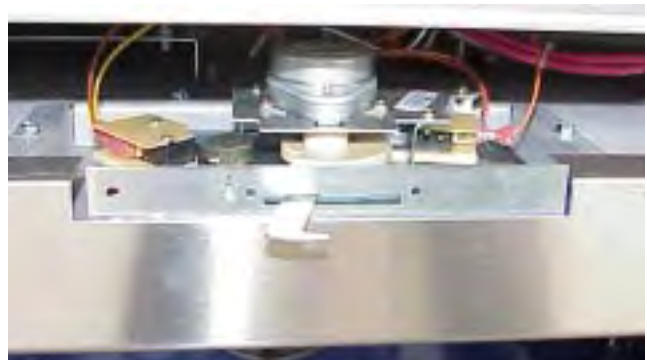
automatic door locking mechanism mounted between the burner box and the top of the oven,
