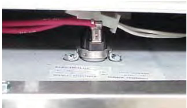
automatic door locking mechanism mounted between the burner box and the top of the oven,
