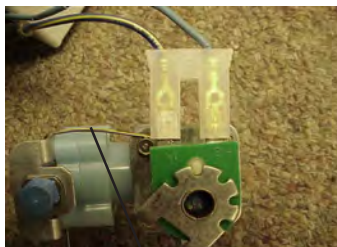
Terminal on Coil is Installed
