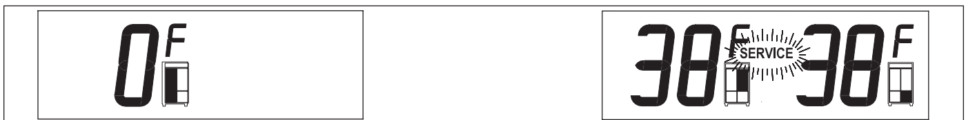
Figure 3-33. "SERVICE" Flashing = Multiple Possibilities; See Error Code History
