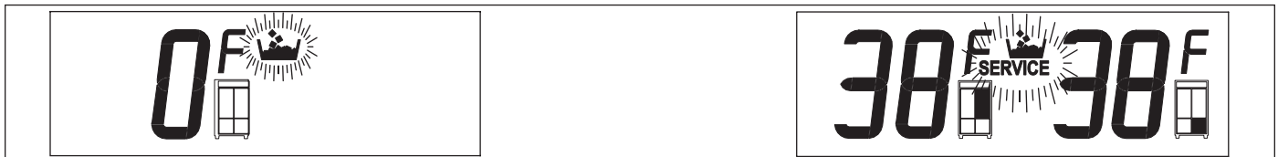
Figure 3-29. ICE & SERVICE Flashing = Solenoid Energized 15 sec., every 12 hrs., 5 Consecutive Times
