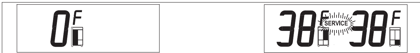
Figure 3-38. “SERVICE” alone Flashing = Multiple Possibilities; See Error Code History
