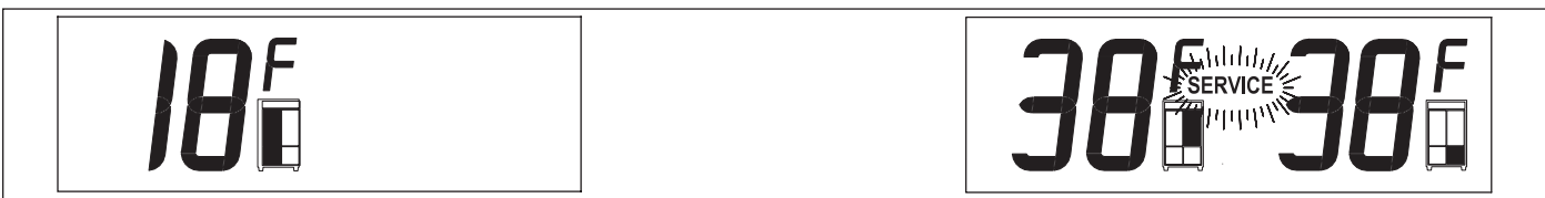
Figure 3-27. SERVICE Flashing = Several Excessive Compressor Run Periods
