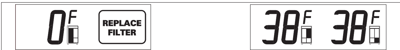
Figure 3-31. REPLACE FILTER Icon Appears after approximately one (1) Year of Filter Use
