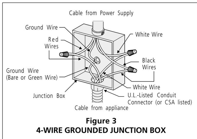
**⚠ CAUTION** If connecting to a 4-wire electrical system, the appliance frame MUST NOT be connected to the neutral wire of the 4-wire electrical system.
