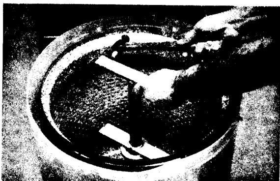
■ USE SPANNER EXTENSION TOOL TO REMOVE NUT
