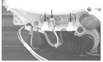
6. Loosen 10mm nut on Heater and remove Heater Element.
