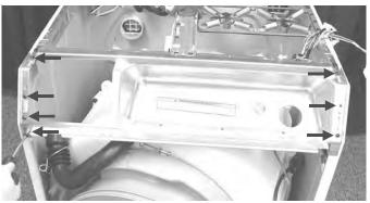
22. Grasp the front and rear of the tub and slide out. Use a blanket or rug to protect the floor
