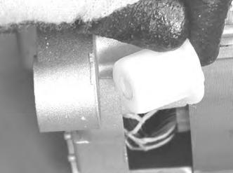
**NOTE:** During reinstallation be sure all four bushings are installed properly
