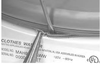
5. Pull the boot from the lip formed into the front opening.
