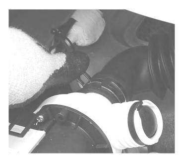
7. Remove screw securing Drain Pump to bracket. Twist Drain Pump clockwise to remove.
