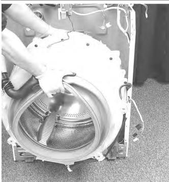
23. Set the tub on the floor. Position 4" wood blocks or equivalent around the spinner shaft. Roll the tub to the upright position and rest it on the blocks.
