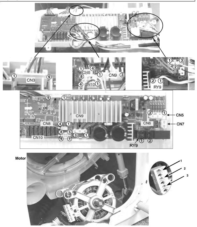
Normal resistance is approximately 3.0? between any 2 pins (1,2 or 3) on motor connector.
