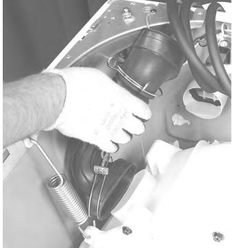
Lift Suspension Spring from keeper in cabinet. Repeat for the opposite side and let Outer Tub rest on support board.
