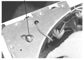
**NOTE:** Mark the wire locations on the EMI before removing the terminals.
