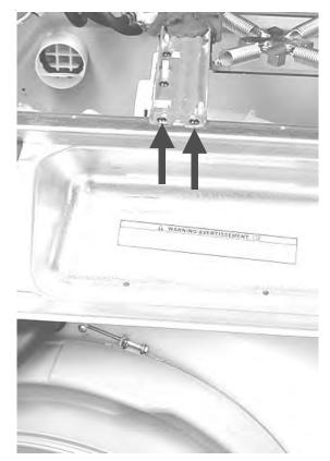
21. Remove remaining screws securing Back Guard to cabinet.
