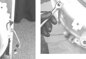
NOTE: Torque tub bolts to 6-11 ft. lbs.
