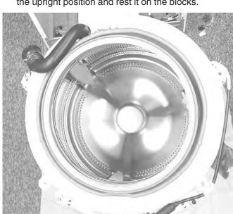
24. Remove the 10mm screws around the perimeter of the tub.
