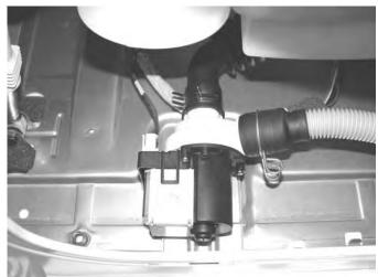
6. Remove three 13mm bolts securing Drain Pump to base.
