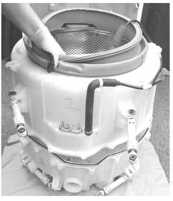
26. Tub Gasket can be replaced after tub halves are split.
